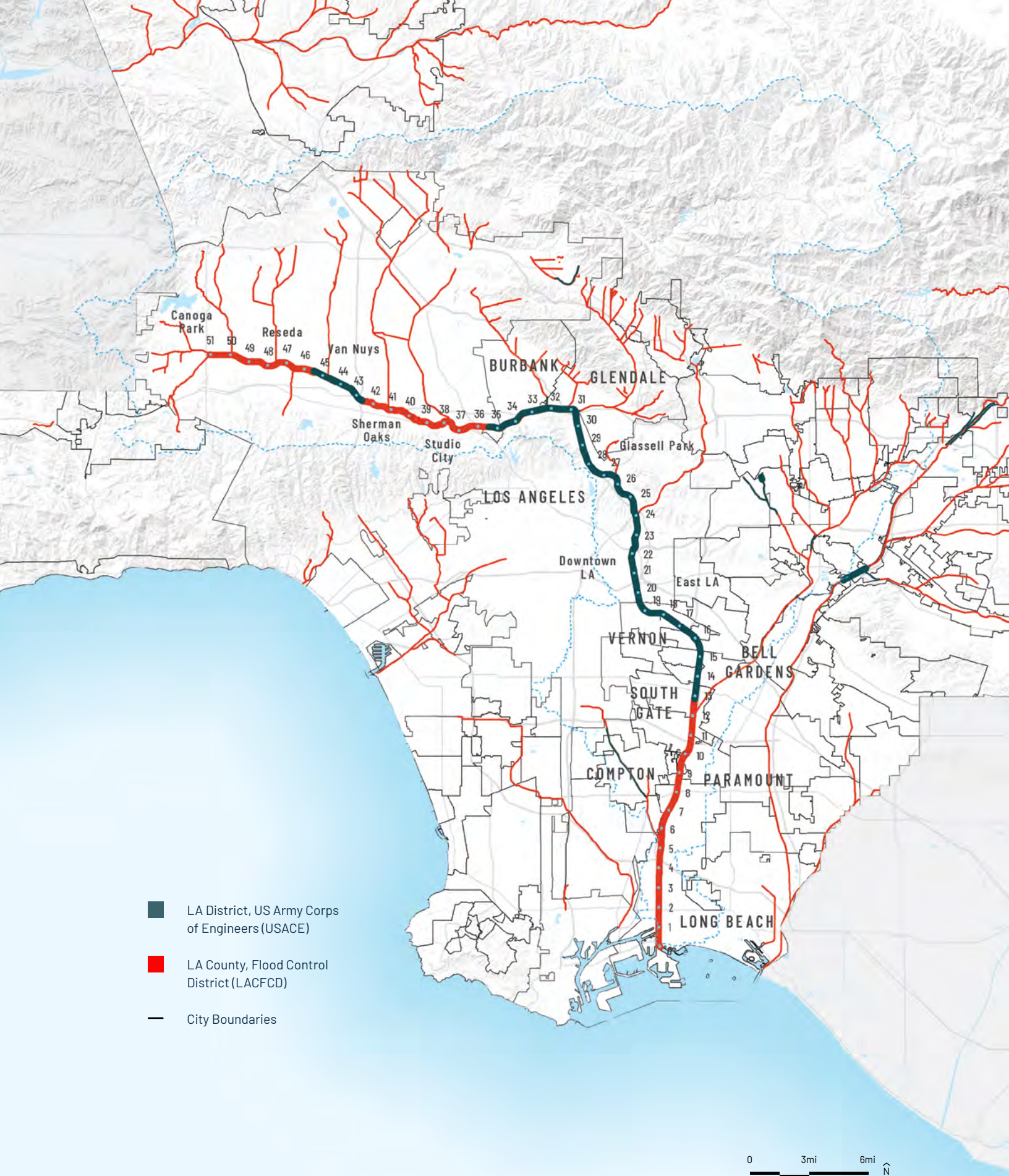
Figure 362. The current operations and maintenance of the LA River and tributaries is shared by the LA County Flood Control District and the US Army Corps of Engineers. Source: LA County GIS Data Portal, City Boundaries and Annexations, 2016, & LA City Communities and Planning Areas, 2014.
