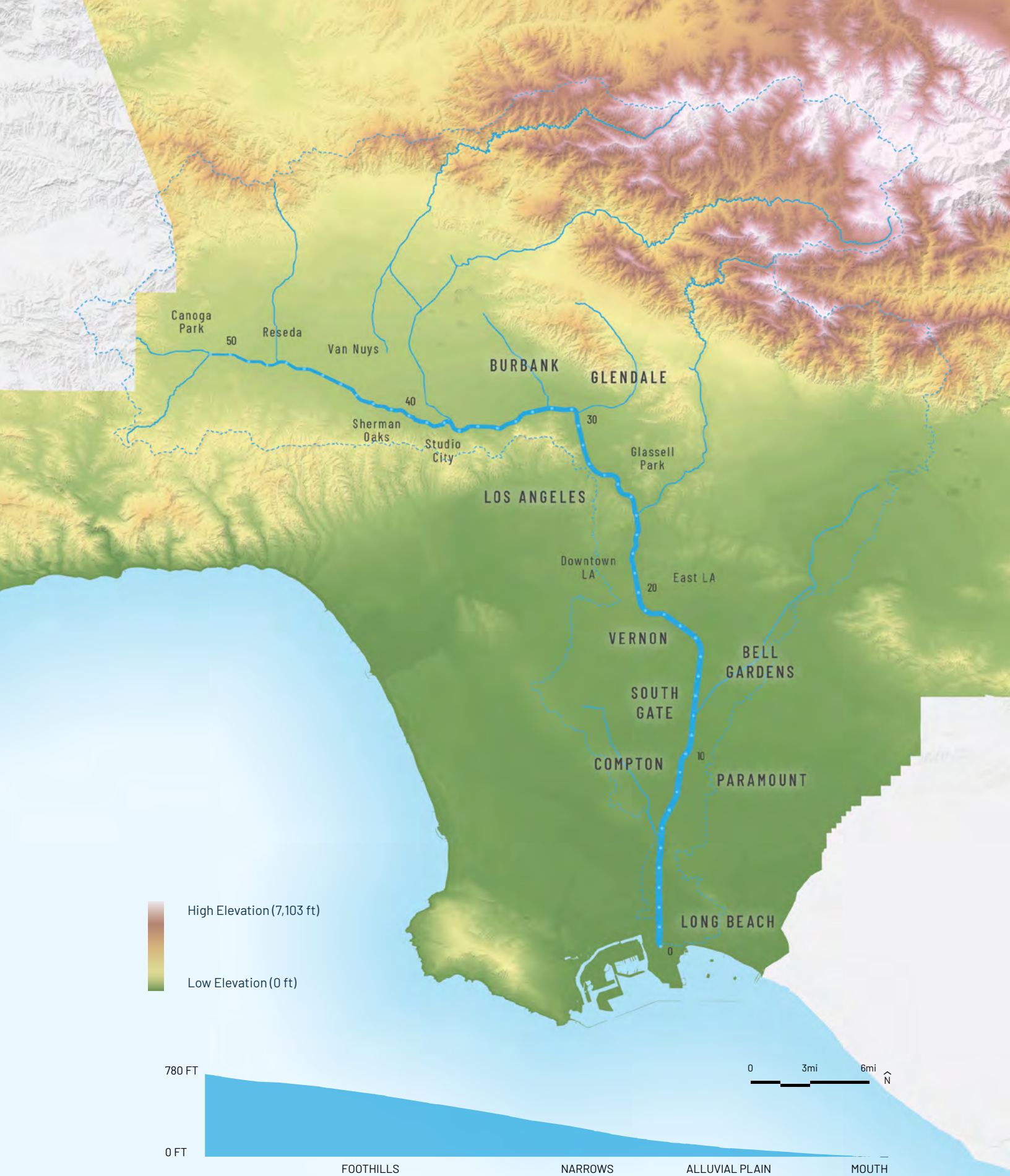
Figure 38. LA County DEM (Digital Elevation Model). The LA River drops 780 feet in just 51 miles. Source: U.S. Geological Survey, 2013; USGS NED 1 arc-second 2013.
