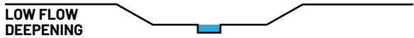
Figure 298. As dry weather flows may decrease in the future, it is desirable to maintain specific beneficial uses along parts of the river. Maintaining beneficial uses during dry weather seasons may require making sections of the low flow channel shallower to allow a smaller volume of water to spread out and maintain habitat, or deeper to maintain recreation opportunities such as kayaking.
