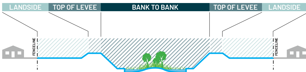
Figure 19. There are a few trapezoidal channel typologies along the LA River. The trapezoidal channel either has a soft or concrete bottom and may or may not have visible levees.
