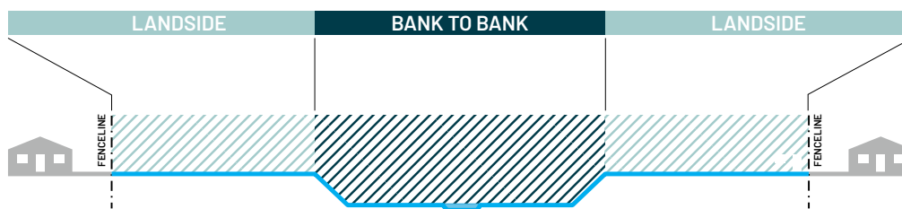
Figure 18. There are two types of channel sections on the LA River: the rectangular box channel and the trapezoidal channel.
